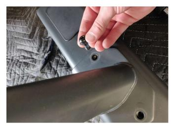
3. Remove stabilizer from the frame and gently let the frame rest on a soft surface.
