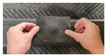
6. Reinstall the stabilizer using the same hardware. Tighten fasteners firmly.
