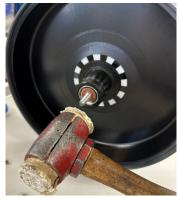
5. Place the axle shaft back into the flywheel from the same direction it came out from. Ensure the axle slides into the inner race of the remaining bearing and use a hammer to tap the end of the axle to knock the remaining bearing out of the flywheel.
