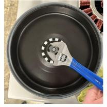
3. Using a 17 mm wrench on the non-drive side jam nut and a 17 mm deep socket on the drive side jam nut, loosen the jam nuts. Only one side will loosen, remove the jam nut on that side.
