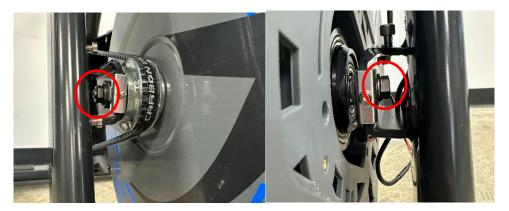
9. Using a 7 mm nut driver, loosen both belt adjuster bolts evenly with the same number of turns. Record the number of turns you loosened the bolts here: \_\_\_\_\_\_ turns each. This will help to keep the flywheel aligned and give a great starting point when you re-tension the belt.
