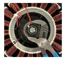
18. While holding the coil assembly inside the flywheel to ensure it does not fall out, flip the flywheel assembly to be driveside up on top of your flywheel support (cylinder or 2x4s). If you are not using a flywheel support, roll a towel up into a circle so the coils are supported by the towel when the flywheel is flipped. Remove the flywheel by lifting it up, the coil assembly will slip out as you lift.
