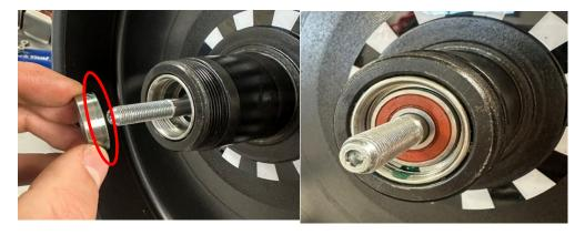
8. Reinstall the bearing cap nut into the flywheel over the bearing and tighten down using the splined cassette tool provided with the repair kit. Torque to 40 Nm (30 lbf-ft).
