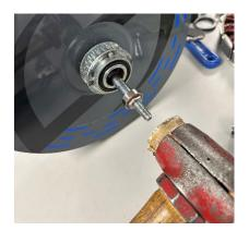
Install a new axle bearing provided with the repair kit onto the <u>drive side</u> axle shaft (drive side of the axle has a <u>shorter</u> inner bearing race shoulder) and then the jam nut. Hand-tighten the jam nut.
