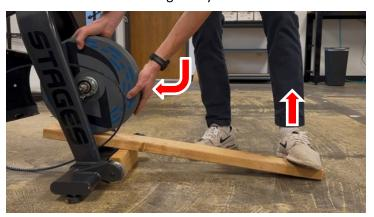
9. Install the flywheel brake stay back into place and tighten the two flywheel anchor bolts using a 5 mm hex key.
