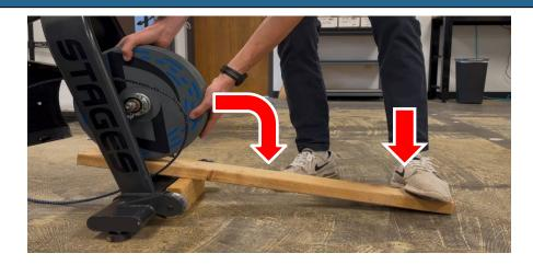
12. Lay the flywheel with the pulley facing down, coils facing up. Since the axle will not allow the flywheel to lay flat, it is recommended to use the two 2x4s to stabilize the flywheel. You can angle the 2x4s to add stability. Another option is to use a hollow cylinder (height between 3 and 6 inches, inner diameter at least 3 inches.)
